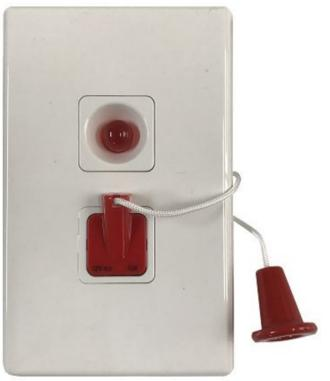
Indigo Care has designed the Pull Cord Pendant with the elderly resident in mind. The call plate is mounted on the ceiling so the resident will have easy access to the pull cord to initiate a call. The cord length can be variable to suit different ceiling heights. There is a red LED for call activity. The switch is momentary action and is reset when the cord is released.
